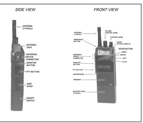
Figure 3 - M-PA Scan Model Radio
